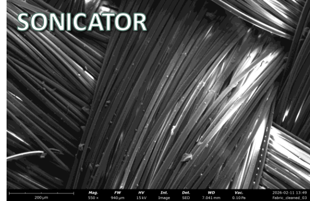
Fig. 8: Ortho-Fabric samples pre- and post-cleaning with various cleaning methods.
