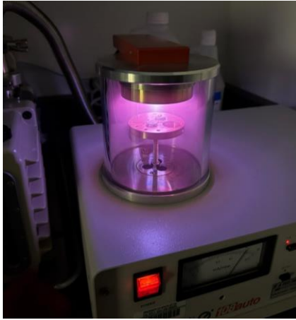
Fig. 6: Gold sputtering non-conductive materials
