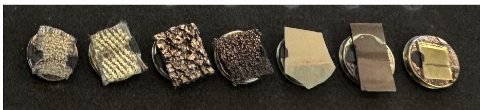
Fig. 6 Mounted and gold-sputtered samples on SEM mounts. Materials from left to right are as follows: OrthoFabric, Nextel fabric, coarse polyurethane foam, fine polyurethane foam, aluminum ceramic, glass, and aluminum.
